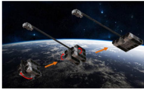
Figure 2.15: View of the re-configuration mechanism of AAReST, also showing the integrated tape spring hinge. (Underwood et al., 2018)
