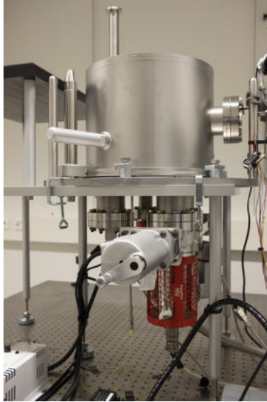
Figure 2.19: Vacuum system on top of its support structure, with ion getter pump (in red) and gate valve visible.
