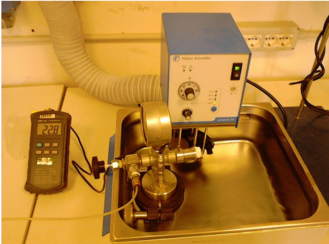
**Figure 3-2 The equipment used for the batch carbonation tests.**
