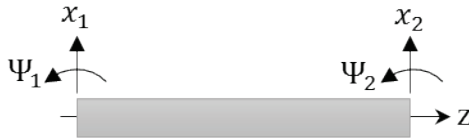
Figure 2: Degrees of freedom of a shaft element in a single plane
